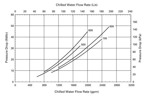
Figure PD-6. ABSD 975-1350 pressure drop vs. chilled water flow rate - English and SI Units
